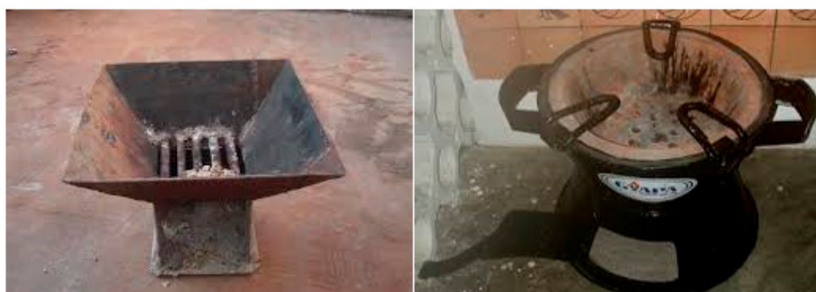
Figure 4. Traditional Coal Pot (Left) and Gyapa Improved Cook Stove (Right) Common the Ghanaian Market.
