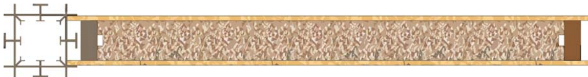
Figure 71. Detail of structural member with SIP panel.
