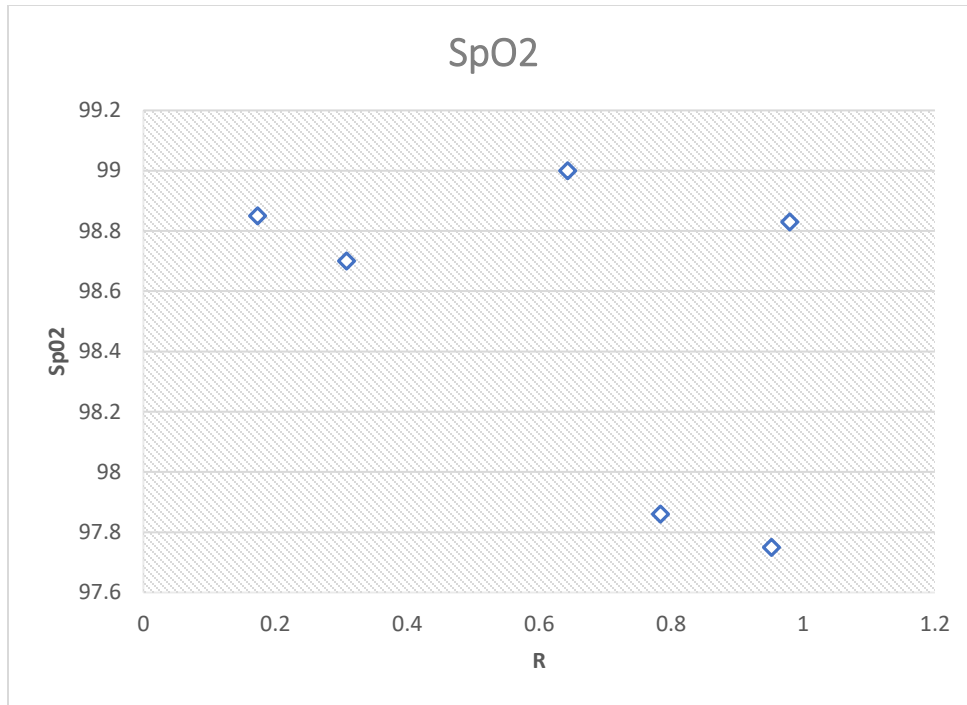
Figure 4.12 Graph between calibrated SpO2 readings vs. calculated R. As SpO2 value tends to increase, ratio R tends to decrease. The two data points where SpO2 is 99 and 98.83 shows certain discrepancies because of the mechanical design of the concave sensor making difficult to collect accurate readings.
