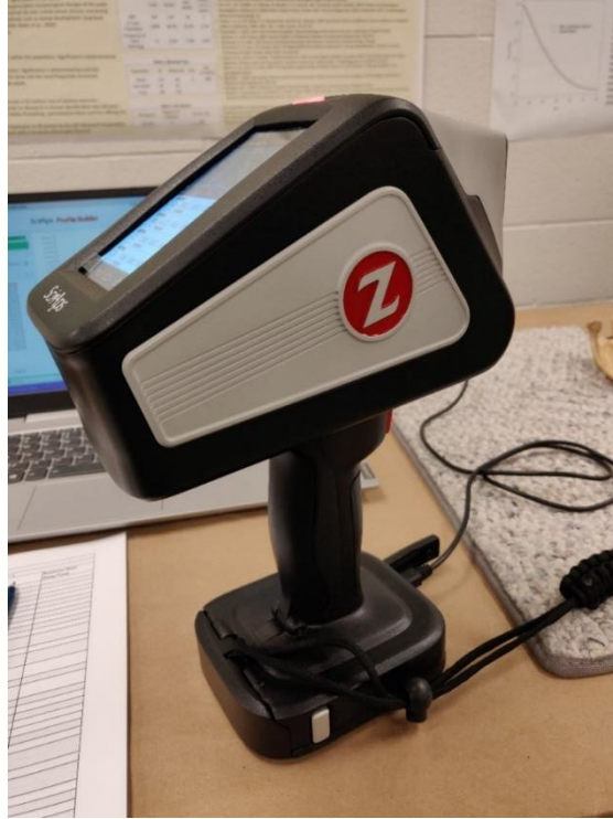
Figure 3.4. SciAps Z-300 handheld LIBS analyzer used for data collection.
