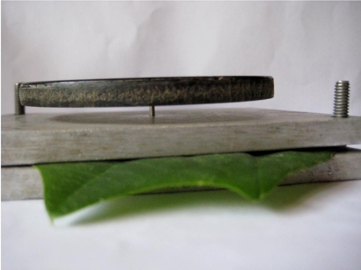
Figure 2. Penetrometer technique used to determine the toughness of each Passiflora leaf sampled.
