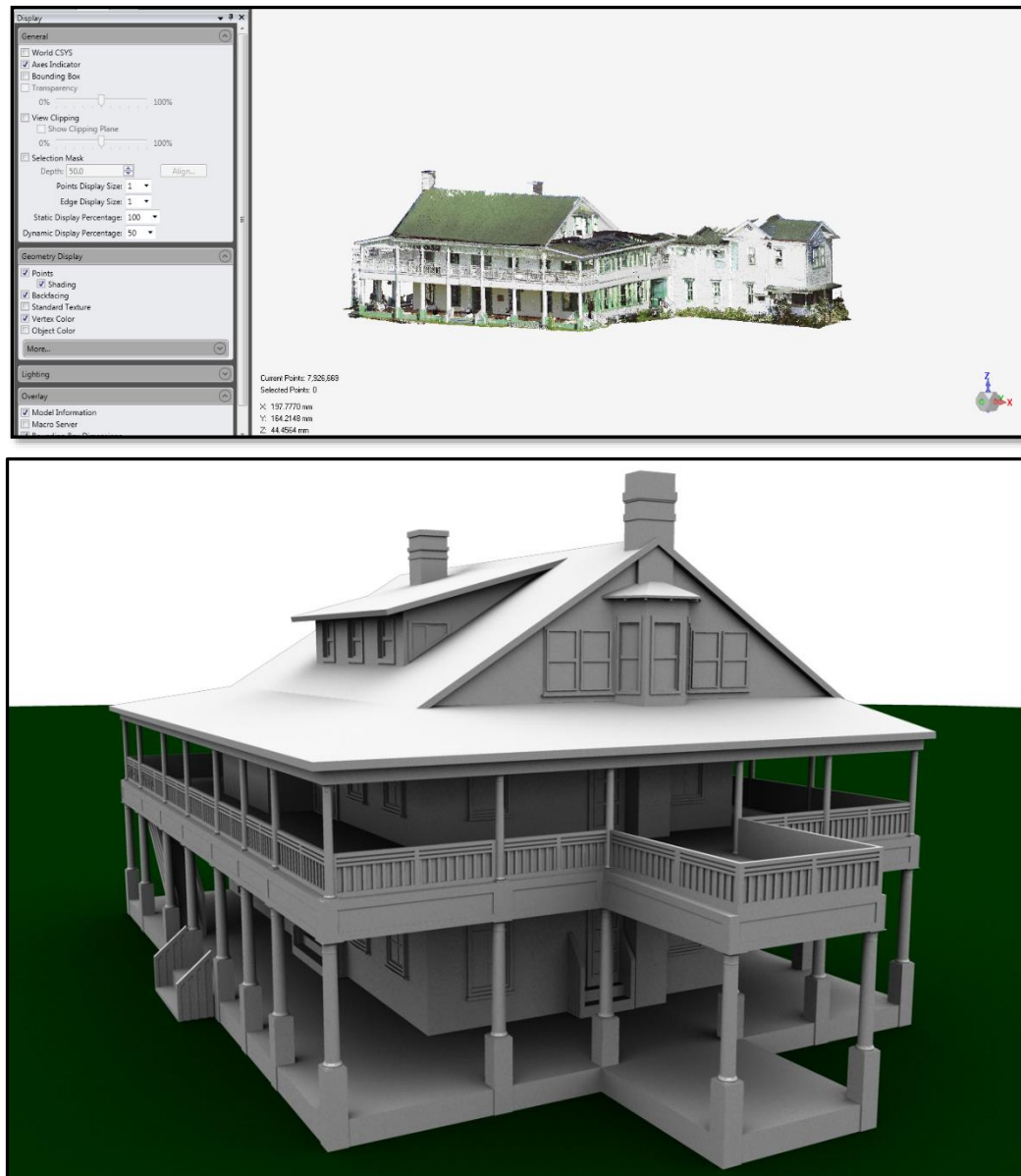
Figure 8. Point cloud of laser scanning data (above) and solid surface 3D CAD render (below) for the Chinsegut Manor House.
