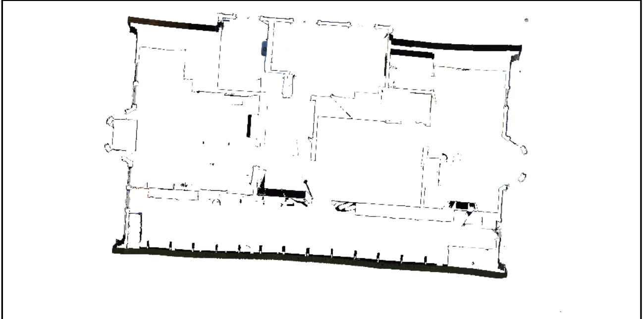
Figure 14. Tomographic slice from laser scan data, showing the third floor. Noted are areas of significant wall deformation and bowing.
