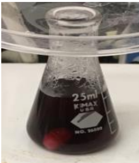
Figure 2. Colloidal Gold Nanoparticle solution. (a) Color changes of solution during course of colloidal AuNPs synthesis with SC as reductant 54 . (b) Color of colloidal gold solution at end of reaction as obtained for this study in our lab.
