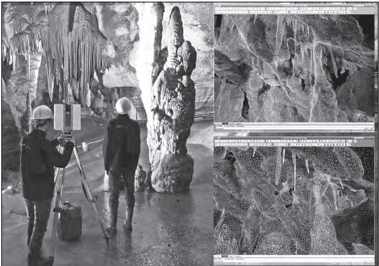
Figure 2: Laser scanning the cave Santa Barbara 1, Iglesias, Italy. Upper right side: a detail of the point cloud of the cave visualized on AutoCAD© platform with Virtualgeo CloudCUBE software. Lower right side: same detail of the 3D model elaborated from the point cloud by using the CloudCUBE 3D modeling functionalities.
