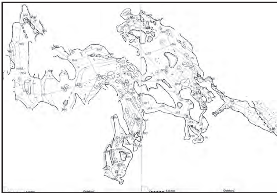
Figure 2: Survey of the Ghale Kord cave (surveyed by the ISEI 2008 team; drawn by Neven Bocic). More than 400 m of underground galleries are surveyed, but the cave is only partially surveyed so far.
