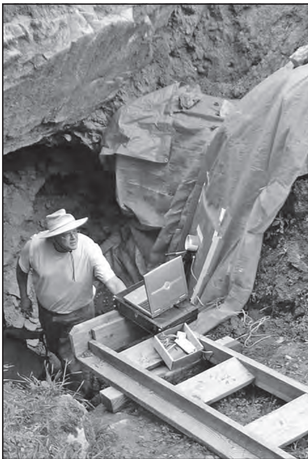
Figure 8: A tarp was fastened to one side of an excavation to cover an area where air was passing through a zone of rocks. Cardboard was taped to the tarp to provide a rigid surface and a hole was cut in the cardboard and tarp. An anemometer was placed in this hole where the air flow was then concentrated.
