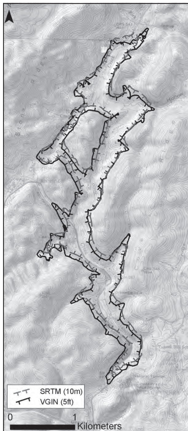
Figure 3: Map of the closed depression at Natural Tunnel State Park, Scott County, Virginia as resolved by contours drawn on a SRTM data-derived DEM and on a high-resolution photogrammetrically-derived terrain model (VGIN).
