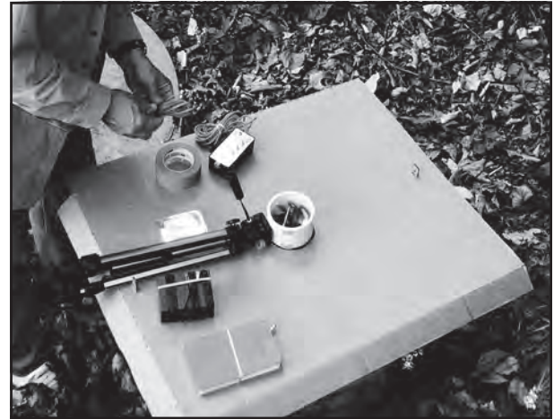
Figure 5: Cardboard has been placed over the entrance (a vertical culvert pipe) to Basswood Cave. The anemometer placed over a hole in the cardboard records the rate of air flow.
