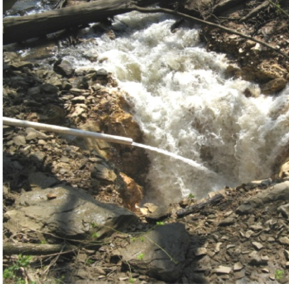
Figure 2. Brine solution addition to the river water recharge to the subsurface conduit.
