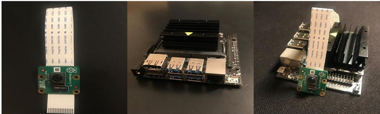
Figure 4 Hardware components shown individually and assembled. Raspberry Pi Camera Module V2 (left), NVIDIA Jetson Nano (middle), unit assembled (right).
