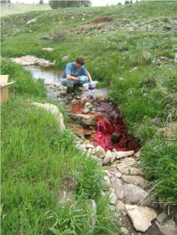
Marc Ohms dumping Rhodamine dye in the newly opened sink point in the bed of Highland Creek. Notice that the sink is capturing the entire flow of Highland Creek at the time of this photo. A month later, the sink started collapsing and water began flowing past the sink. June 2008. Photo by Rod Horrocks.
