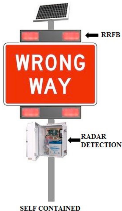
Fig. 1. Red RRFBs mounted on “WRONG WAY” sign (Recreated from WUSF News, 2015)
